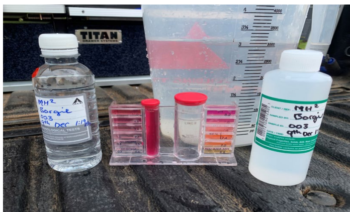
Samples collected and sent off for bacteriological testing Mourquong Water main Extension
