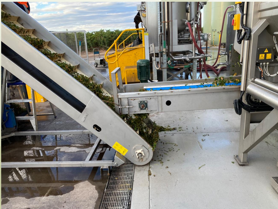
Figure 2 Leaves and stem separated before being crushed
