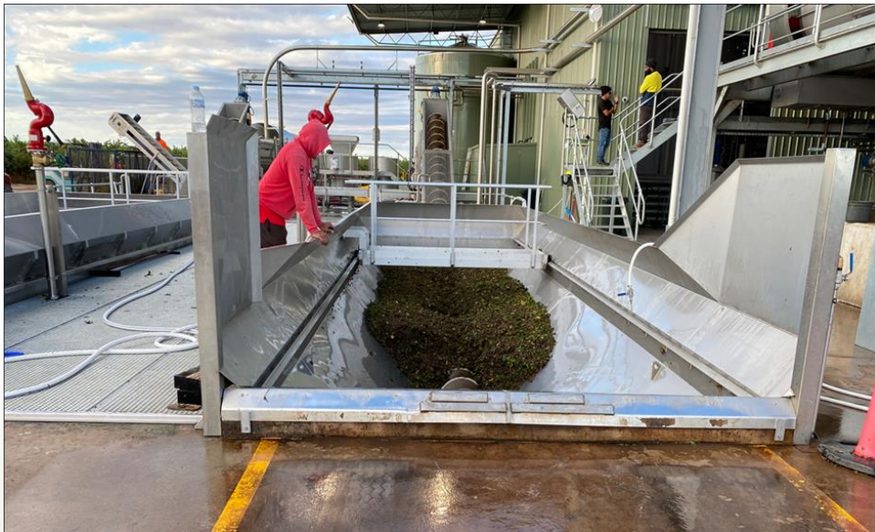
Figure 1 Grapes being moved using an auger in the bin
