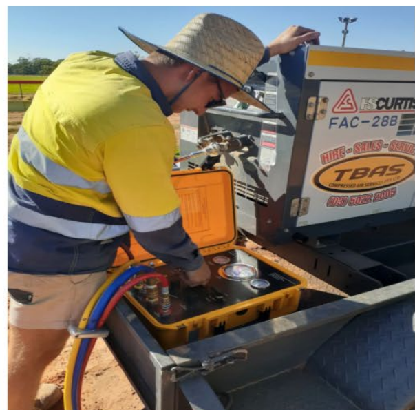
Setup of testing gauges – 24/02/2022)
