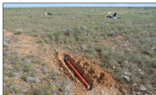
A geophysicist at an MT site. A vertical magnetic field sensor in the background and a horizontal sensor (~1.5 m long) in the foreground.
