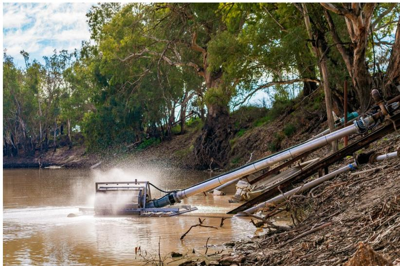
*Figure 1: The 8 inch Riverscreen floating diversion screen operating at Porker Citrus on the Darling River at Ellerslie. (Image: David Sickerdick Photography)*
