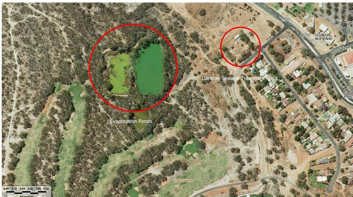
*Figure 1* - Shows the Dareton wastewater treatment plant location and the evaporation ponds for the plant effluent. The red circles denote the area likely to be affected in the event of a sewage off site release.
