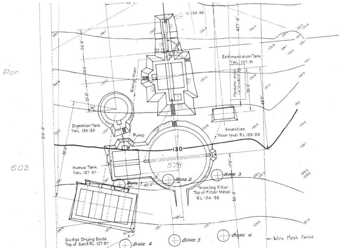
Figure 2 - shows the location of potential pollutants on the site. Sedimentation tank on the top contains untreated sewage, the filter in the middle contains untreated sewage, the humus tank to the left contains treated effluent and the digester on the right contains digested sludge.
